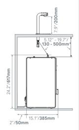
\* Hosing should be trimmed to ensure continuous drop from font to boiler
